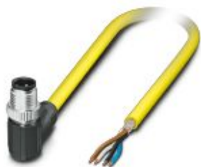
Sensor/actuator cable, 4-position, PVC, yellow, shielded, Plug angled M12, coding: A, on free cable end, cable length: 10 m
