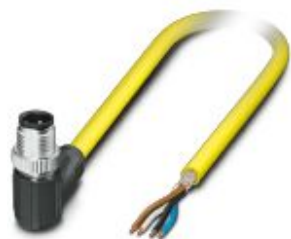
Sensor/actuator cable, 4-position, PVC, yellow, shielded, Plug angled M12, coding: A, on free cable end, cable length: 5 m
