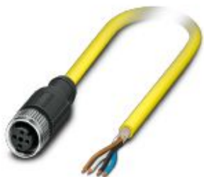
Sensor/actuator cable, 4-position, PVC, yellow, shielded, free cable end, on Socket straight M12, coding: A, cable length: 5 m
