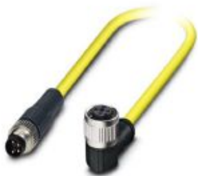
Sensor/actuator cable, 4-position, PVC, yellow, Plug straight M8, on Socket angled M12 SPEEDCON, coding: A, cable length: 1.5 m
