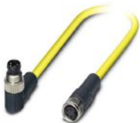
Sensor/actuator cable, 4-position, PVC, yellow, Plug angled M8, on Socket straight M8, cable length: 0.5 m
