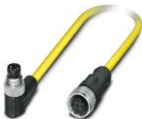
Sensor/actuator cable, 4-position, PVC, yellow, Plug angled M8, on Socket straight M12 SPEEDCON, coding: A, cable length: 0.5 m
