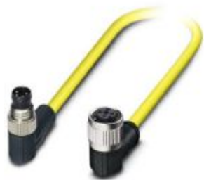
Sensor/actuator cable, 4-position, PVC, yellow, Plug angled M8, on Socket angled M12 SPEEDCON, coding: A, cable length: 1.5 m
