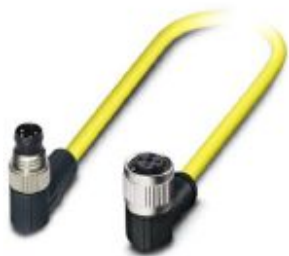
Sensor/actuator cable, 4-position, PVC, yellow, Plug angled M8, on Socket angled M12 SPEEDCON, coding: A, cable length: 0.5 m
