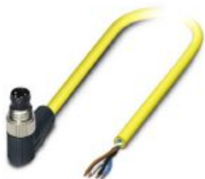
Sensor/actuator cable, 4-position, PVC, yellow, Plug angled M8, on free cable end, cable length: 10 m
