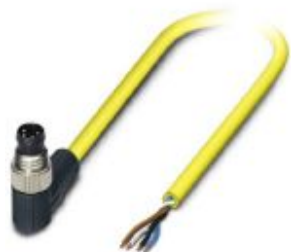
Sensor/actuator cable, 4-position, PVC, yellow, Plug angled M8, on free cable end, cable length: 2 m
