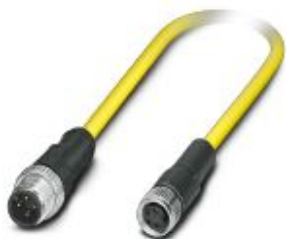
Sensor/actuator cable, 4-position, PVC, yellow, Plug straight M12 SPEEDCON, coding: A, on Socket straight M8, cable length: 1.5 m
