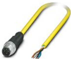
Sensor/actuator cable, 4-position, PVC, yellow, Plug straight M12, coding: A, on free cable end, cable length: 5 m
