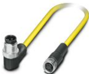
Sensor/actuator cable, 4-position, PVC, yellow, Plug angled M12 SPEEDCON, coding: A, on Socket straight M8, cable length: 1.5 m
