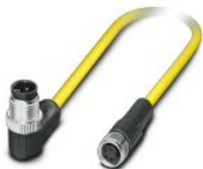
Sensor/actuator cable, 4-position, PVC, yellow, Plug angled M12 SPEEDCON, coding: A, on Socket straight M8, cable length: 0.5 m
