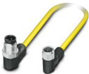
Sensor/actuator cable, 4-position, PVC, yellow, Plug angled M12 SPEEDCON, coding: A, on Socket angled M8, cable length: 0.5 m
