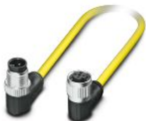
Sensor/actuator cable, 4-position, PVC, yellow, Plug angled M12, coding: A, on Socket angled M12, coding: A, cable length: 1.5 m
