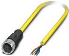
Sensor/actuator cable, 4-position, PVC, yellow, free cable end, on Socket straight M12, coding: A, cable length: 5 m
