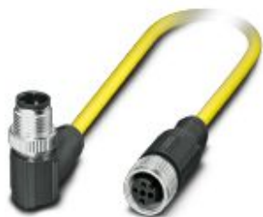
Sensor/actuator cable, 3-position, PVC, yellow, shielded, Plug angled M12, coding: A, on Socket straight M12, coding: A, cable length: 0.5 m
