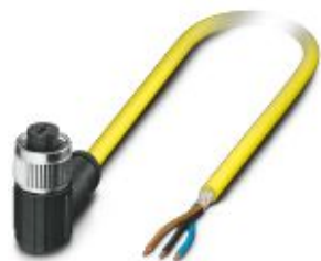
Sensor/actuator cable, 3-position, PVC, yellow, shielded, free cable end, on Socket angled M12, coding: A, cable length: 5 m
