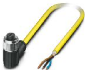
Sensor/actuator cable, 3-position, PVC, yellow, shielded, free cable end, on Socket angled M12, coding: A, cable length: 2 m
