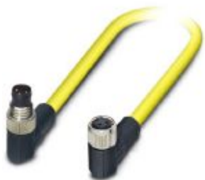
Sensor/actuator cable, 3-position, PVC, yellow, Plug angled M8, on Socket angled M8, cable length: 1.5 m
