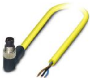
Sensor/actuator cable, 3-position, PVC, yellow, Plug angled M8, on free cable end, cable length: 2 m
