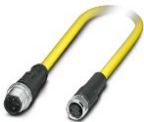
Sensor/actuator cable, 3-position, PVC, yellow, Plug straight M12, coding: A, on Socket straight M8, cable length: 1.5 m
