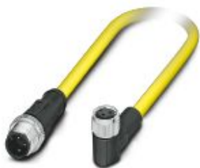
Sensor/actuator cable, 3-position, PVC, yellow, Plug straight M12, coding: A, on Socket angled M8, cable length: 1.5 m
