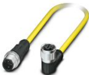
Sensor/actuator cable, 3-position, PVC, yellow, Plug straight M12, coding: A, on Socket angled M12, coding: A, cable length: 0.5 m
