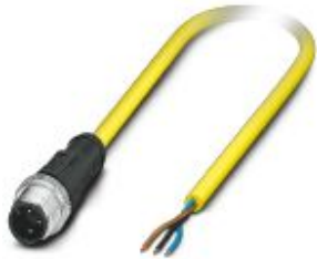
Sensor/actuator cable, 3-position, PVC, yellow, Plug straight M12, coding: A, on free cable end, cable length: 10 m
