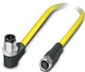
Sensor/actuator cable, 3-position, PVC, yellow, Plug angled M12, coding: A, on Socket straight M8, cable length: 1.5 m
