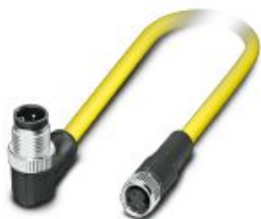
Sensor/actuator cable, 3-position, PVC, yellow, Plug angled M12, coding: A, on Socket straight M8, cable length: 0.5 m
