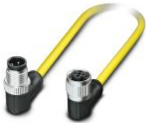
Sensor/actuator cable, 3-position, PVC, yellow, Plug angled M12, coding: A, on Socket angled M12, coding: A, cable length: 0.5 m
