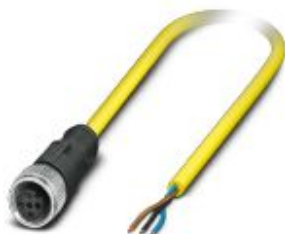
Sensor/actuator cable, 3-position, PVC, yellow, free cable end, on Socket straight M12, coding: A, cable length: 5 m
