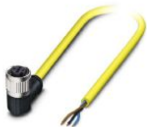
Sensor/actuator cable, 3-position, PVC, yellow, free cable end, on Socket angled M12, coding: A, cable length: 2 m
