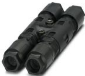
QUICKON H-distributor, black, 4 pos. +PE, 1.0 mm 2 ... 2.5 mm 2 / 690 V / 20 A, for cable diameters of 9 mm ... 16 mm, with a sealing bolt.
