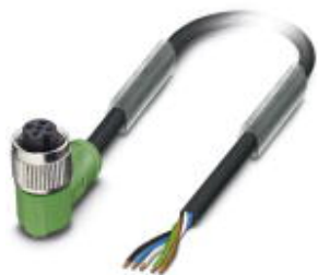
Sensor/actuator cable, 5-position, PVC, gray RAL 7001, free cable end, on Socket angled M12, B-coded, cable length: 5 m
