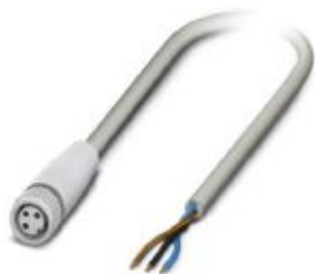
Sensor/actuator cable, 3-position, PP-EPDM halogen-free, gray RAL 7035, free cable end, on Socket straight M8, cable length: 1.5 m, Hygienic design, with plastic knurl
