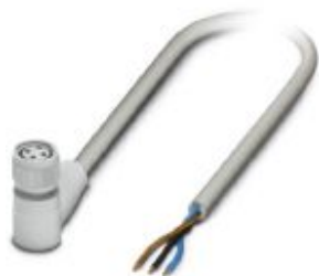
Sensor/actuator cable, 3-position, PP-EPDM halogen-free, gray RAL 7035, free cable end, on Socket angled M8, with 2 LEDs, cable length: 1.5 m, Hygienic design, with plastic knurl
