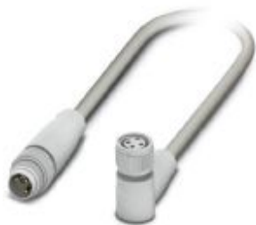
Sensor/actuator cable, 3-position, PP-EPDM halogen-free, gray RAL 7035, Plug straight M8, on Socket angled M8, with 2 LEDs, cable length: 0.3 m, Hygienic design, with plastic knurl
