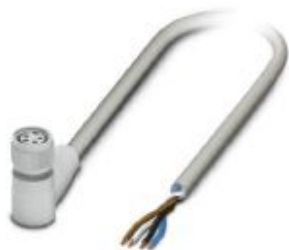
Sensor/actuator cable, 4-position, PP-EPDM halogen-free, gray RAL 7035, free cable end, on Socket angled M8, with 2 LEDs, cable length: 3 m, Hygienic design, with plastic knurl
