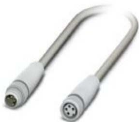
Sensor/actuator cable, 4-position, PP-EPDM halogen-free, gray RAL 7035, Plug straight M8, on Socket straight M8, cable length: 0.6 m, Hygienic design, with plastic knurl
