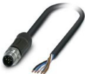
Sensor/actuator cable, 5-position, PE-X halogen-free, black-gray RAL 7021, Plug straight M12, coding: A, on free cable end, cable length: 10 m, for outdoor applications, with high-grade steel knurl
