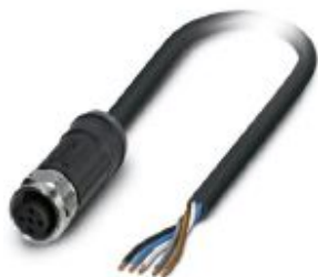
Sensor/actuator cable, 5-position, PE-X halogen-free, black-gray RAL 7021, free cable end, on Socket straight M12, coding: A, cable length: 2 m, for outdoor applications, with high-grade steel knurl
