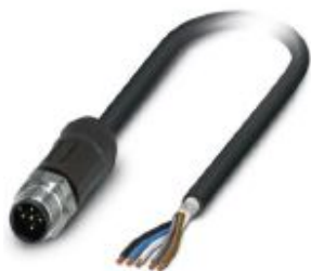
Sensor/actuator cable, 5-position, PE-X/PE-X halogen-free, black-gray RAL 7021, shielded, Plug straight M12, coding: A, on free cable end, cable length: 10 m, for outdoor applications, with high-grade steel knurl
