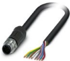
Sensor/actuator cable, 8-position, PE-X halogen-free, black-gray RAL 7021, Plug straight M12, coding: A, on free cable end, cable length: 10 m, for outdoor applications, with high-grade steel knurl
