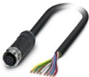
Sensor/actuator cable, 8-position, PE-X halogen-free, black-gray RAL 7021, free cable end, on Socket straight M12, coding: A, cable length: 2 m, for outdoor applications, with high-grade steel knurl
