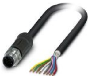
Sensor/actuator cable, 8-position, PE-X/PE-X halogen-free, black-gray RAL 7021, shielded, Plug straight M12, coding: A, on free cable end, cable length: 10 m, for outdoor applications, with high-grade steel knurl
