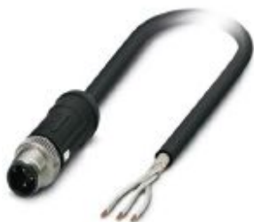
Sensor/actuator cable, 3-position, PE-X halogen-free, black, shielded, Plug straight M12 SPEEDCON, coding: A, on free cable end, cable length: 10 m, For railway applications
