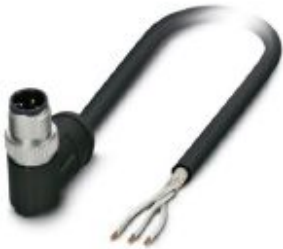
Sensor/actuator cable, 3-position, PE-X halogen-free, black, shielded, Plug angled M12 SPEEDCON, coding: A, on free cable end, cable length: 5 m, For railway applications
