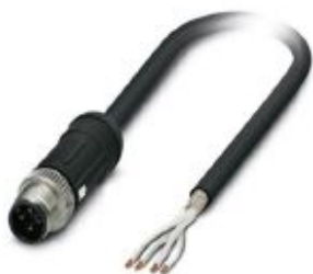
Sensor/actuator cable, 4-position, PE-X halogen-free, black, shielded, Plug straight M12 SPEEDCON, coding: A, on free cable end, cable length: 2 m, For railway applications
