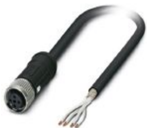
Sensor/actuator cable, 4-position, PE-X halogen-free, black, shielded, free cable end, on Socket straight M12 SPEEDCON, coding: A, cable length: 2 m, For railway applications
