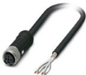
Sensor/actuator cable, 4-position, PE-X halogen-free, black, shielded, free cable end, on Socket straight M12 SPEEDCON, coding: A, cable length: 10 m, For railway applications
