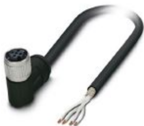
Sensor/actuator cable, 4-position, PE-X halogen-free, black, shielded, free cable end, on Socket angled M12 SPEEDCON, coding: A, cable length: 10 m, For railway applications
